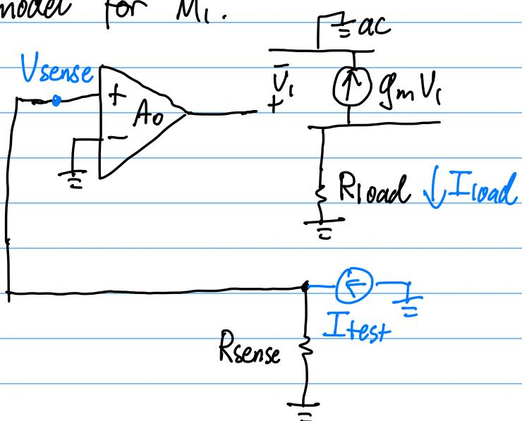
$$V_{sense} = I_{test} R_{sense}$$
