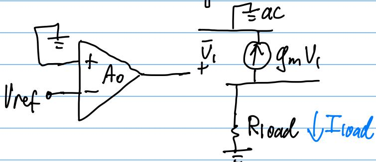
$$V_1 = -A_o V_{\text{ref}}$$
