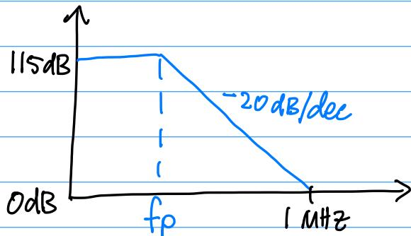
$$\text{There are } \frac{115 \text{ dB}}{20 \text{ dB/dec}} = 5.75 \text{ decades between } f_p \text{ and } 1 \text{ MHz.}$$
