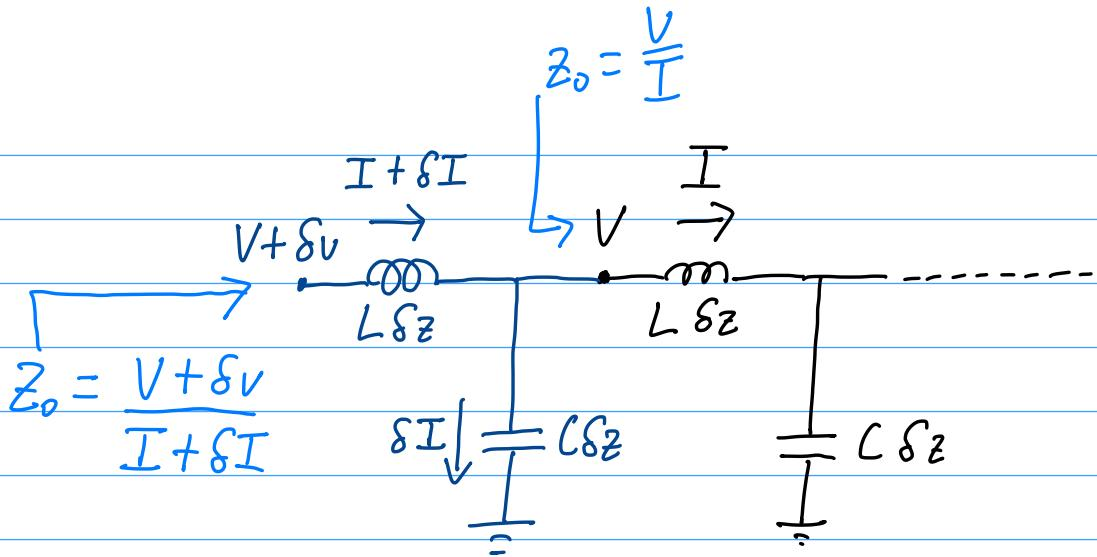
$$(a) \quad Z_c = \frac{1}{j\omega C \delta z} \quad \therefore \delta I = \frac{V}{Z_c} = j\omega C \delta z \quad V$$
