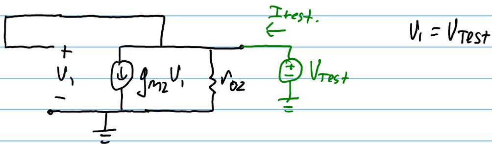
By KCL:  $I_{test} = g_m V_{test} + \frac{V_{test}}{r_{o1}} = (g_m + \frac{1}{r_{o1}}) V_{test}$
