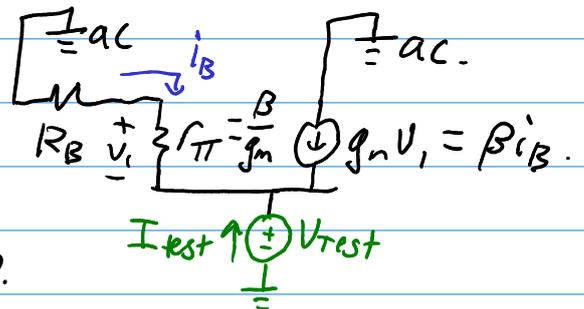
By KCL,  $i_B + I_{test} + \beta i_B = 0$
