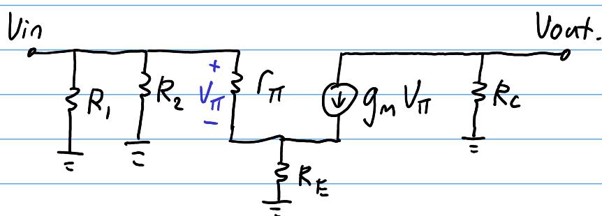
Output impedance is defined with  $V_{in} = 0 \therefore V_{pi} = 0$
