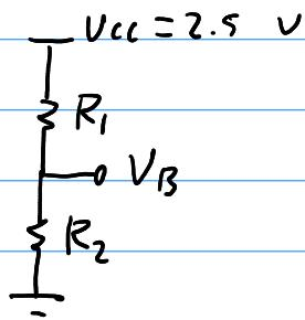
$$V_B = \frac{V_{CC} R_2}{R_1 + R_2}$$
