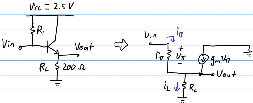
$$\text{By KCL at } V_{out}: i_L = i_B + g_m V_{\pi}$$
