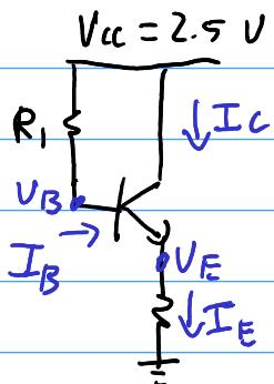
$$\begin{aligned} R_1 &= \frac{V_{CC} - V_B}{I_B} \\ &= \frac{V_{CC} - V_B}{I_C/\beta} \\ &= 221.1 \text{ k}\Omega \end{aligned}$$
