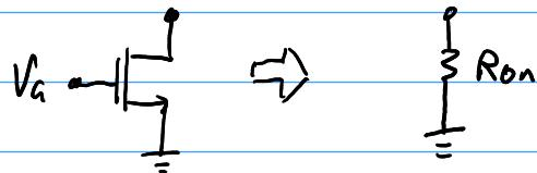
Since the supply voltage is 1.8 V, we could choose  $V_{AS}$  in the range  $0 \leq V_{AS} \leq 1.8 V$ .
