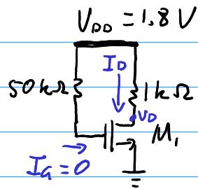
Given  $M_1 C_{ox} = 200 \frac{mA}{V^2}$ ,  $\lambda = 0$ ,  $V_{TH} = 0.4 V$ .
