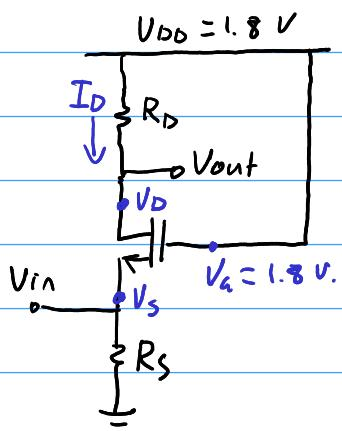
$$I_D = \frac{P}{V_{DD}} = \frac{0.002}{1.8} = 1.11 \text{ mA.}$$
